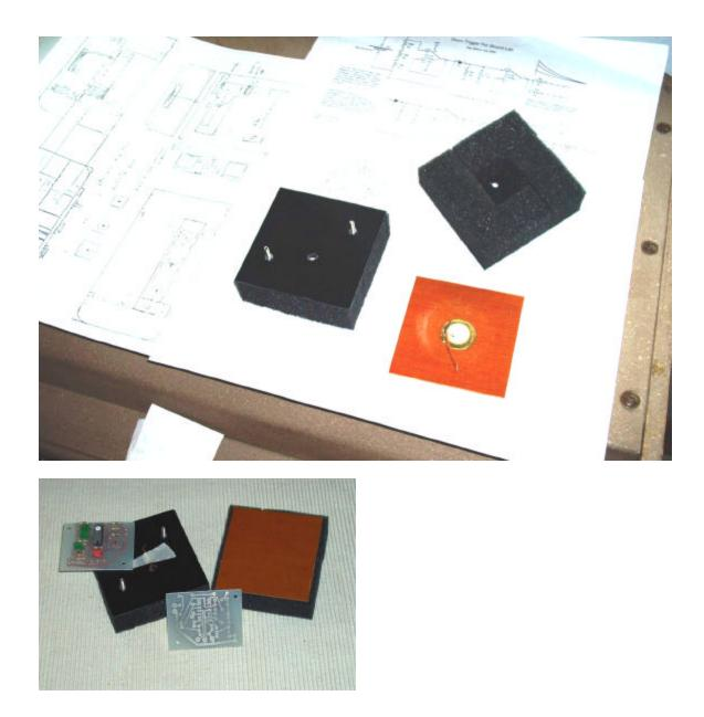
The populated PCB gets mounted to the module on the studs after all the external wiring is in place. Note that the thin element wires got a drop of silicone adhesive to keep them from being yanked out of the piezo element:
