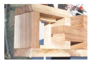
The above photo provides another view of how the pieces were assembled. The 5/16" pieces were mounted so that two provided a stop for the drum trigger modules. These are glued 1 9/16" from the top edge of each drum. The second two were glued 1/16" from the bottom edge of each drum to provide a mounting point for the bottom covers. The  $\frac{1}{4}$ " X  $\frac{1}{4}$ " groove is clearly visible in this shot.
