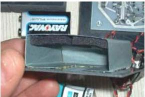
The batteries needed to be isolated from the pcb and jack terminals. I formed this simple holder from fish paper (a stiff paperboard with good dielectric properties) and glued it to the plastic cover for the bottom of the drum with contact cement. Scrap paperboard – think cereal box- would work just as well. Some foam was added to the inside of this holder with silicone cement. This will keep the batteries from rattling around.
