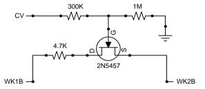
When the gate from the 10 step sequencer is applied the WSG's filter will be modulated by a preset attack-decay provided by the selected network. Switch up gives a WUP-WUP effect. Switch down gives a CO-CO effect. The gate switches on the 10 step sequencer allow you to hear the step or not.
