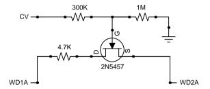
Input 0 to 9V to modulate the frequency of the Voice A Wacky Oscillator. Higher voltage higher frequency lower voltage lower frequency.
