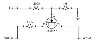
Input 0 to 9V to modulate the frequency of the Voice B Wierd Oscillator. Higher voltage higher frequency lower voltage lower frequency.
