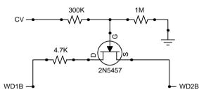
Input 0 to 9V to modulate the frequency of the Voice B Wacky Oscillator. Higher voltage higher frequency lower voltage lower frequency.
