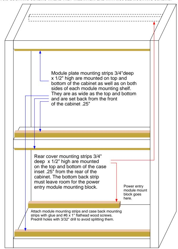
AVOID LOCATING SCREWS WHERE THEY WILL INTERFERE WITH MODULE MOUNTING SCREWS!
