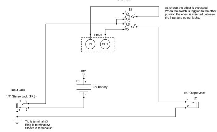
When mono guitar jack is inserted the ring and sleeve are connected together by the jack's sleeve. Thus the battery minus terminal is connected to the PC board's GND input and the effect is powered.
