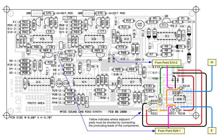
Inverted level shifted outputs now go to the front panel as point "W" and point "E"
